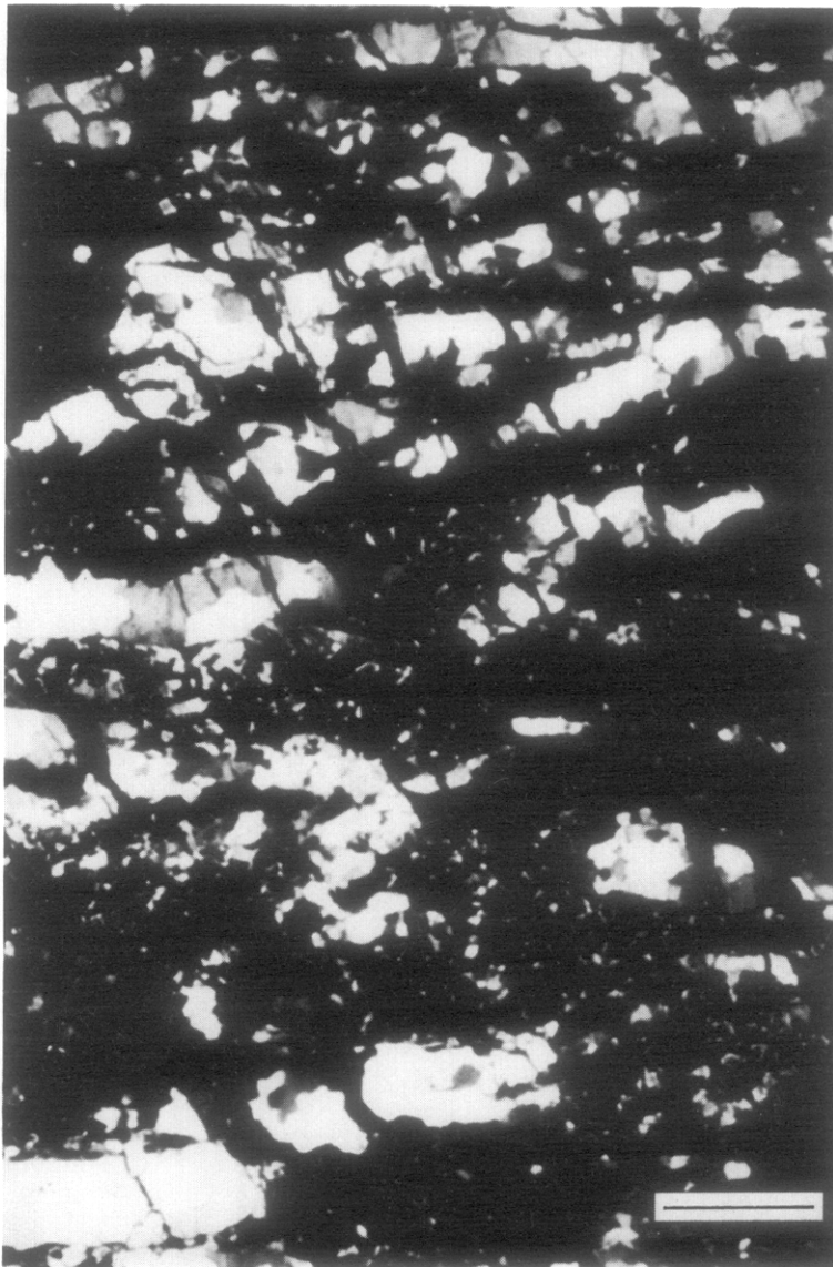
Fig. 2. Fabric of the Harry Creek Pseudotachylytes illustrating the relict ribbon-quartz aggregates of the parent blastomylonitic fabric. Dark regions are melt domains. Crossed nicols. Scale bar is 1mm.
